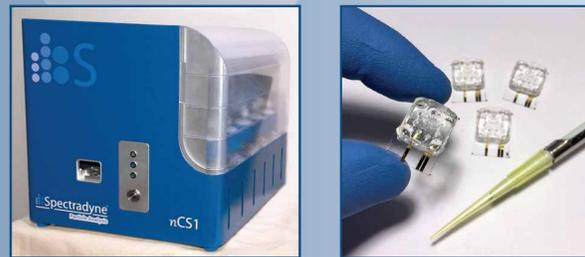
The Spectradyne nCS1 is a compact instrument (left) occupying only 1 linear foot of bench space. Only 3 μL of a sample is required for analysis in a disposable microfluidic cartridge (right), which eliminates contamination and cleaning requirements.
