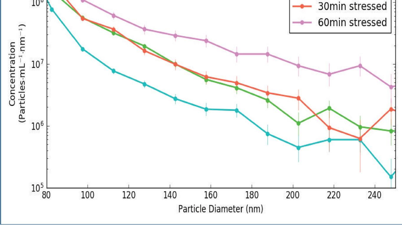
Generally, a clear trend of increasing particle concentration with increasing stress time was observed over the full range of measured diameters. The relative change for small diameters, however, increased significantly more than for large diameters, as shown in Figure 2.
