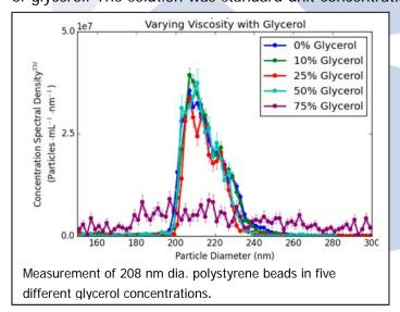
with glycerol concentrations ranging from 0% up to 75%. The corresponding viscosities are displayed in the table. In each measurement, the nCS1
