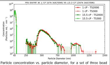
diameters (50, 500 and 1000 nm), measured in two different sucrose concentrations. The measurements overlay exactly, showing the independence of nCS1's RPS measurement method to viscosity.
