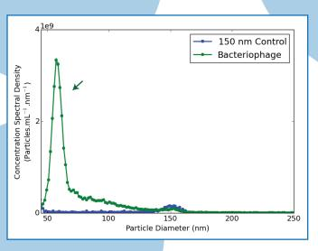
The nCS1's ability to characterize nanoparticles that have index of refraction close to that of the surrounding medium makes it well suited for the quantitative analysis of biological nanoparticles such as virus. In addition, the high resolution concentration-size distributions delivered by the nCS1 provide a new opportunity to quantify polydispersity in situ in complex biological samples—a capability that has until now not been available in a commercial instrument.
